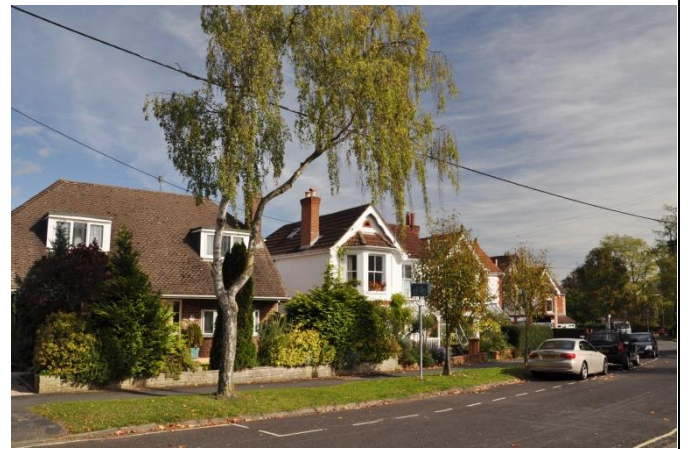
Figure 2C-10 Looking east further east along the street from photo number 27. Note to the right of the view the pre-war development of houses on the north side with gabled fronts, bay windows, ornate bargeboards and stonework/brickwork quoins. The sequence starts with number 10, the rendered white painted house
